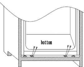
Fit the seal to the appliance, cut off the excessive part if necessary. Fit the bottom parts with plastic covers.
