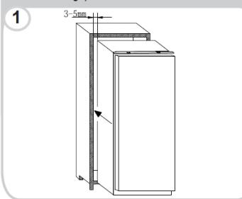
After ensuring the match between appliance door and column door, then screw the appliance upper part to the cabinet
