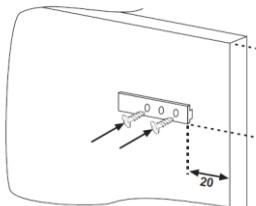
Open the doors of the built-in column and the fridge. Position the built-in loader in the slide, then fit it into the fridge door.
