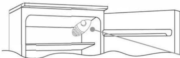
The thermostat box to control the appliance is located inside the fridge compartment on the top right. To check whether the appliance is functioning, make sure that the thermostat knob is not set on "0".
